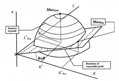
coordinate axis of the production factor labour L(K=0) and RoR - r > 0 represents the tangent of the angle, which the plane of boundary forms with the positive half-axis K. The bounding plane intersects the elipsoid of the values of the profit of the firm, whereby the points below this plane and on this plane represent the profit allowable under the regulation and the points above this plane the non-allowable profit of the firm.
